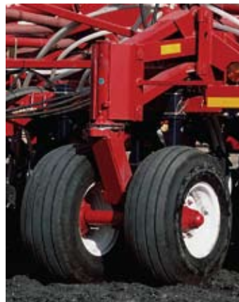
Dual casters on the front gauge wheels ensure a smooth, even ride.
