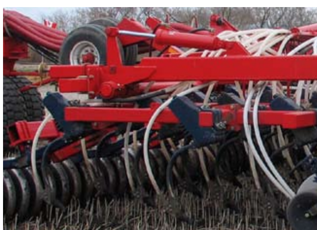
Only Morris' trip reduces pressure as it lifts higher minimizing stress on shanks, trip components and the frame.
