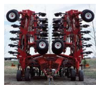
Low profile distribution on the five frame Maxim III allows for a tight, compact transport.
