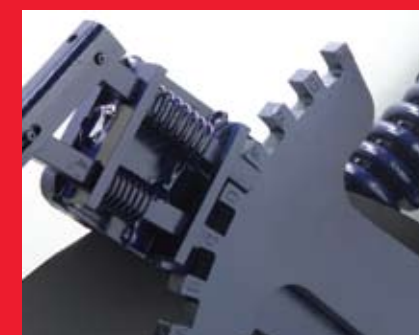
Fertilizer depth is controlled by the soil retaining wheel and a simple ratchet assembly for precise incremental adjustment.
