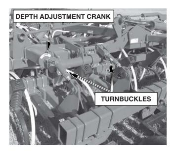
Note: Any change in the depth setting can now be done by adjusting all the depth adjustment cranks evenly across the whole unit. (See Depth Adjustment)
