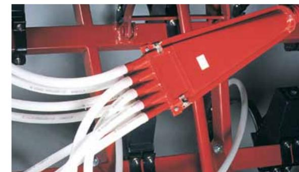
Patented Flat Fan Divider Heads maintain the smooth horizontal flow of product as it leaves the primary runs to divide into each secondary run. The abrupt directional changes, common to vertical divider head systems, are eliminated. This results in an accurate and efficient air delivery system that is exceptionally gentle on your seed. Germination, growth and vigor are protected.
