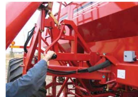
A 10" orbital drive auger is double hinged for exceptional balance and manoeuvrability. Alignment pins lock the auger for extra stability. Top auger lighting is standard.
