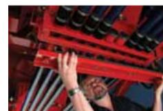
Remove the bottom panel to allow product to flow past the collector directly into the hopper for a quick and simple clean out.
