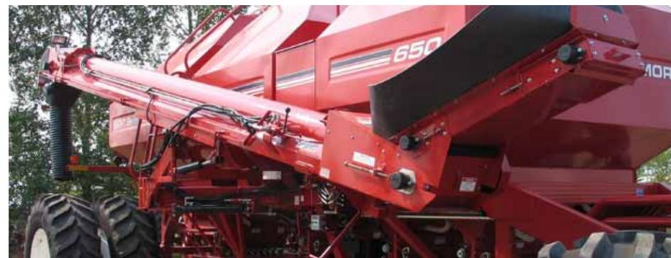
Optional conveyor for 8435, 8630 and 8650 models features a fast 60 bushel per minute loading time with hydraulic remote for convenient one-person operation and requires no clean-out.
