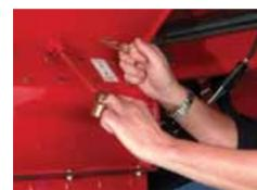
Slide shut-offs on all three tanks provide access to the meter components without having to empty product from the tanks.
