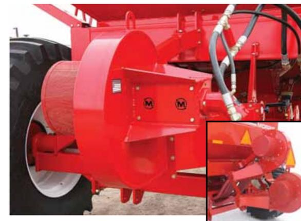
An industrial piston-type hydraulic motor powers a 17" diameter forward curved fan that is 98% efficient. The larger hydraulic lines decrease flow restrictions for less heat build-up under higher fan speeds. A dual fan option for large width seeding tools is available.
