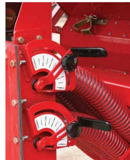
A fully adjustable plenum lets you divert more air to the meter with heavier products and higher rates of application, and less with lighter or more fragile products
