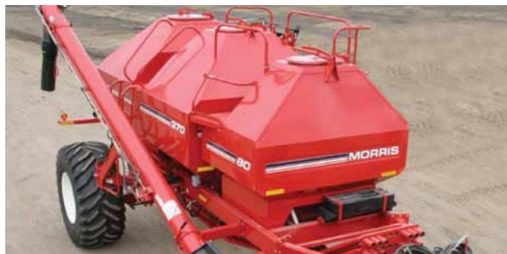
A spacious catwalk design provides safe, convenient access to all tanks at once. Sure grip ladders on both sides fold up out of the way when not in use.
