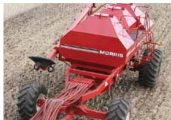
The 8435, 8630 8650 EIGHT Series XL air carts feature a quad steer chassis – using larger tires on the front of the air cart allows you to reduce tire pressure and therefore reduce soil compaction.
