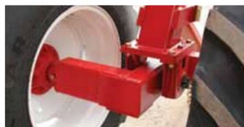
Large offset front tires with walking axles increase stability on corners, side hills and in transport, resulting in a smoother overall ride.
