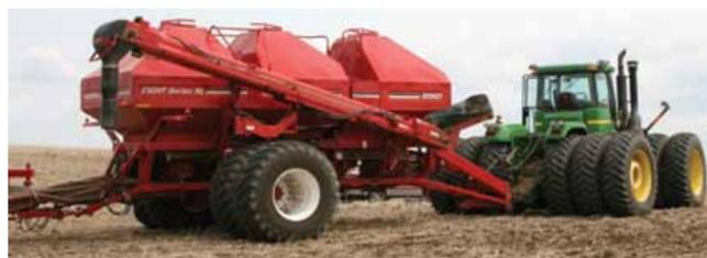
On the tow-between 8650 model the forward axle design provides better weight distribution, lower hitch weight and a tighter turning radius. High floatation, heavy duty dual 800 tires ensures excellent carrying capacity and reduces soil compaction.
