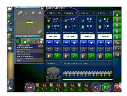
TIP: we use an abbreviation of the word Canola, this because when the tanks are collapsed on the SEEDER-HOME screen the names become shortened. CANOLA-BLEND would appear as CANOLA... Thus causing confusion as to which is the SEED and which is the Fertilizer.
