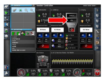
16. Press the Open Tank Fill Window.
