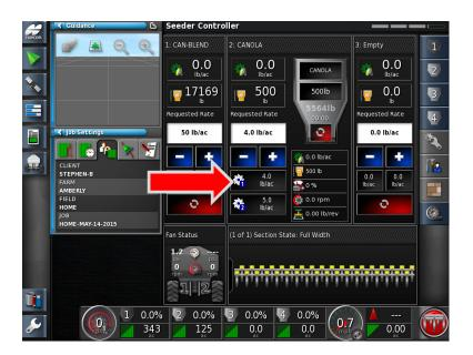
20. Tank 2: has been filled with the desired product CANOLA. Press the Request Application Rate Preset 1 to use the default preset information. Note: The requested Rate window now shows 4.0lb/ac.
