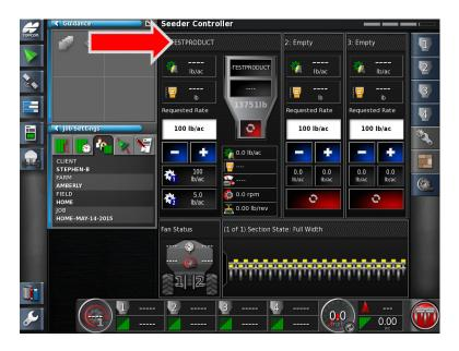
3. Expand the Tank you wish to add the Product into by pressing on the top Band.
