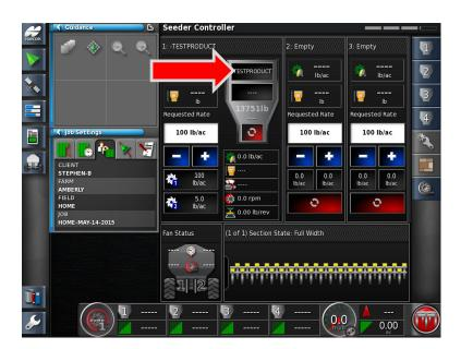
4. Press on the **Top Area** of the Tank – to open the Product Configuration Window.
