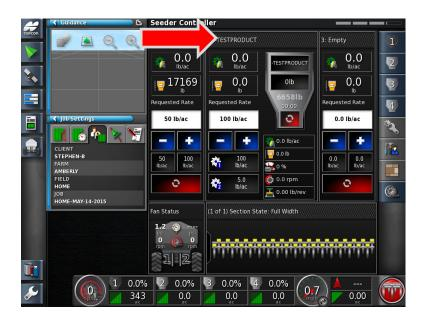
10. Minimize Tank 1 and Expand Tank 2.
