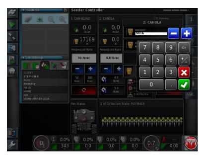
18. Using the keypad enter the Weight manually. Proceed by pressing the Green Check mark.
