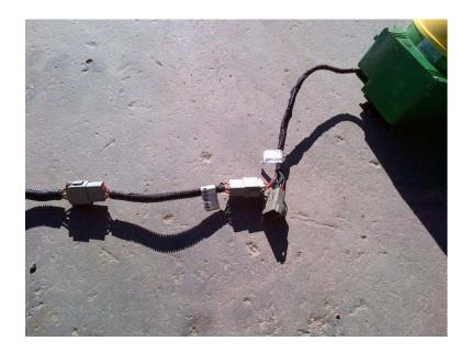
1. Attach **PFP10470** to the female end of StarFire 3000 antenna. Connect the remaining end of PFP10470 to the longer plug on the **PF80754 Y-Harness**.
