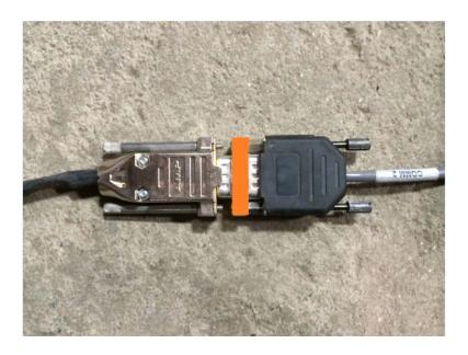
3. Attach an **Orange mini M/M Null Modem** adapter between **the PF80754 serial connector** and the **COMM 2 input** on the X30 AGA5072 harness.
