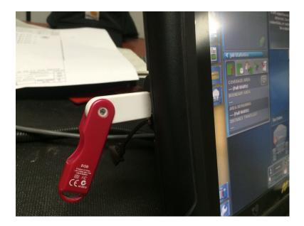
23. Insert the Master Profile List USB stick into the side of the X30 monitor.
