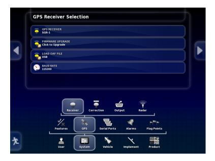
20. Navigate from **System-GPS- Receiver**. Select the Type of GPS antenna you will be using. The default entry level antenna which is included with the X30 is the SGR-1.
