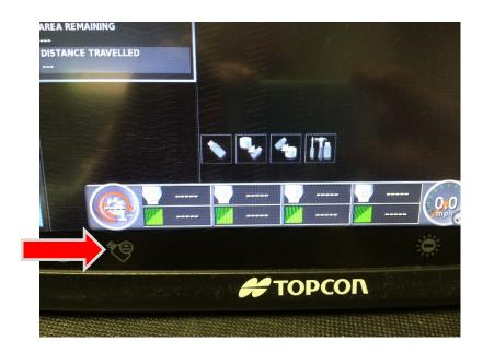
31. At this time it would best to remove the USB memory stick. Press the **USB Eject Icon** on the bottom left of the monitor.
