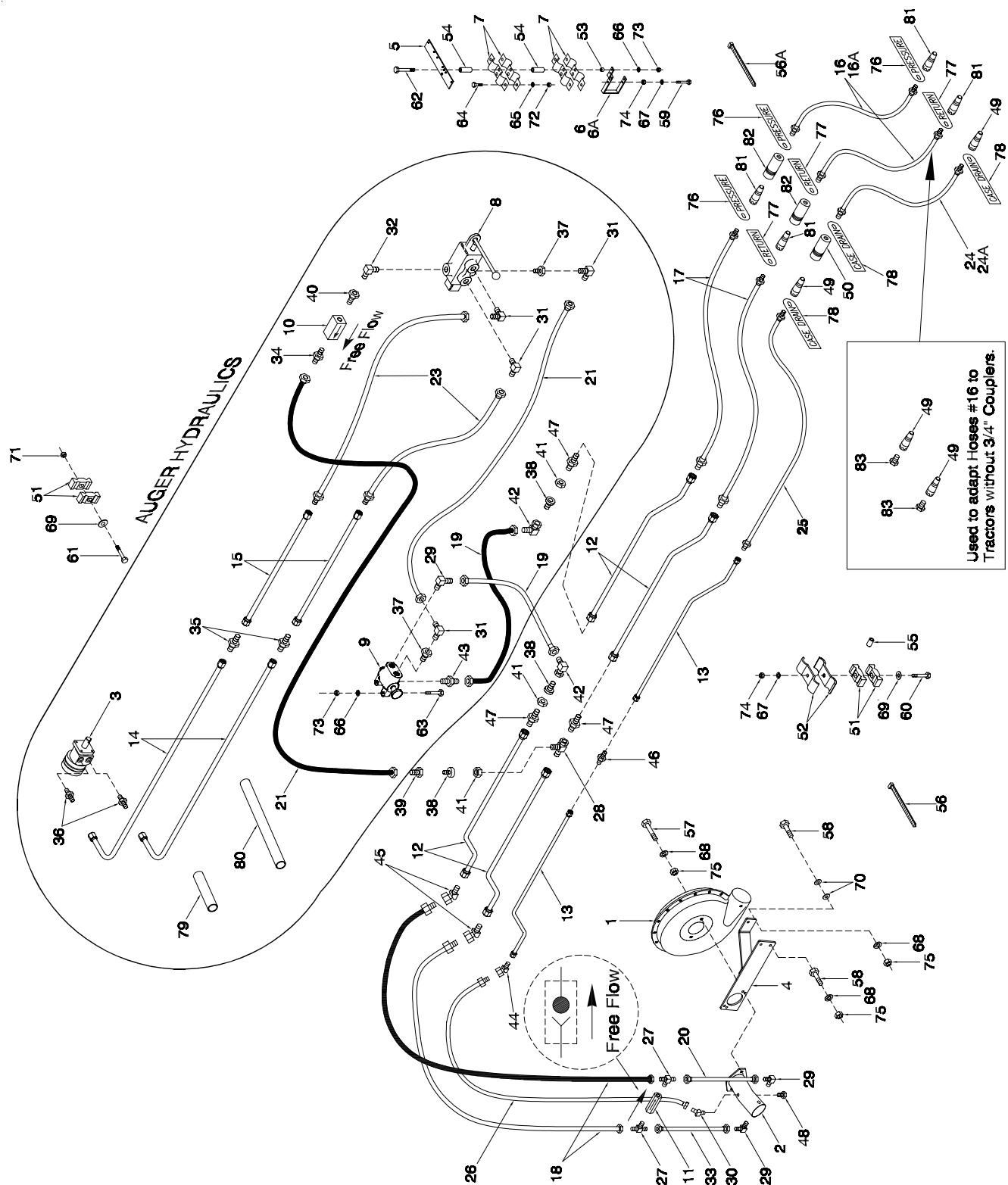
**Fan & Auger Drives- Tow Behind Hydraulic Drive w/Auger (From December 2004)**
