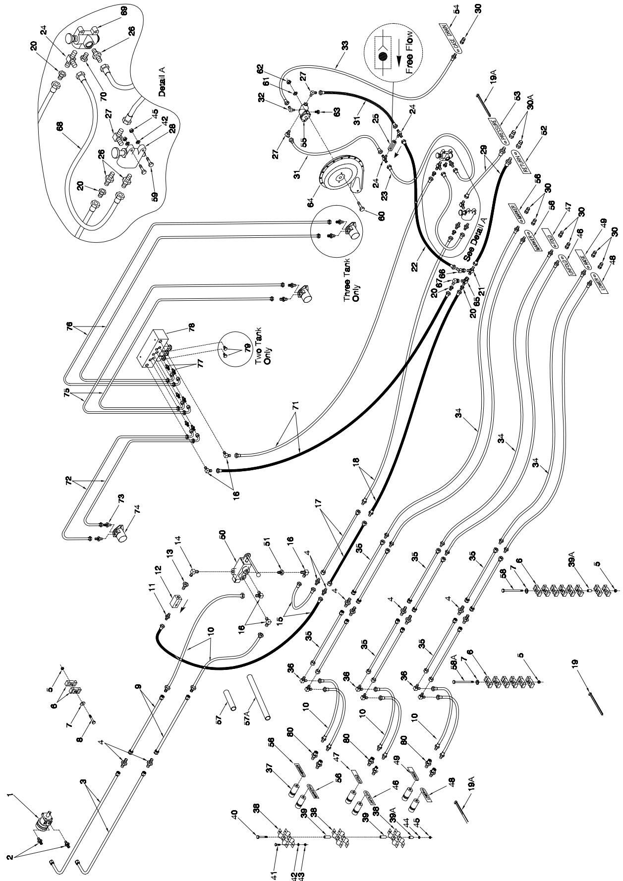
**Variable Rate System- Tow Between Hydraulic Drive w/Auger (From December 2004)**
