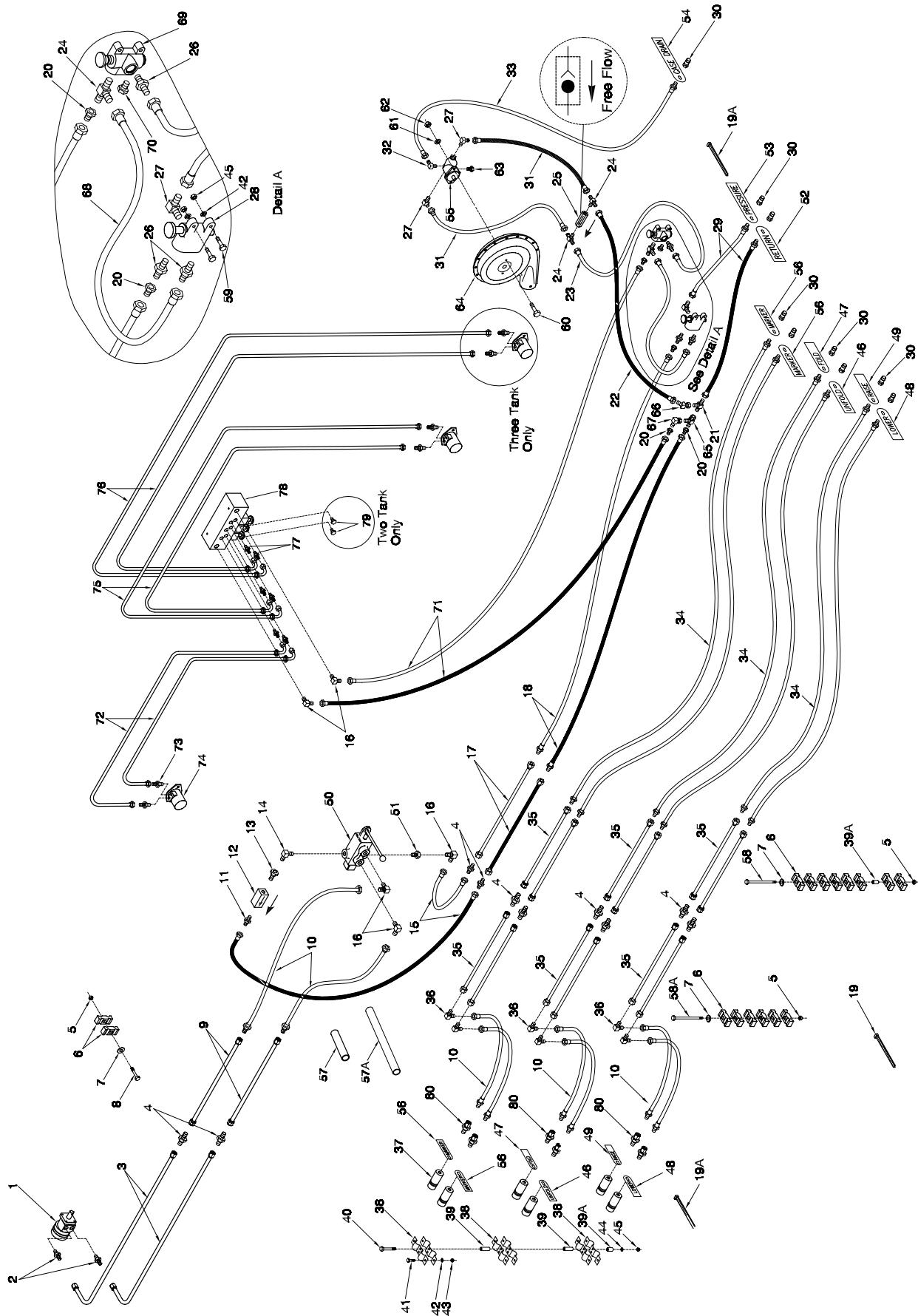
**Variable Rate System- Tow Between Hydraulic Drive w/Auger (Prior to December 2004)**
