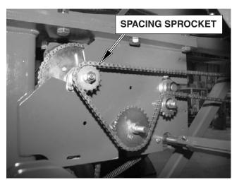
**Spacing Sprocket inside of Left Rear Frame**
