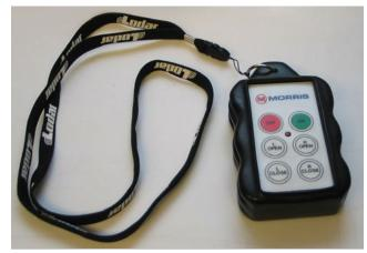
Meter Shut-Off Remote Control
