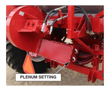
Set Plenum Damper so that setting is in the middle of slot.
