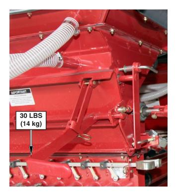
Adjust the latch bolts to obtain a force of 30 lbs (14 kg) to close the Door.
