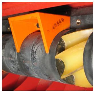
Correctly Installed Blank Off
