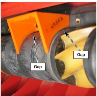
Incorrectly Installed Blank Off
