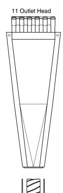
11 Outlet Metering Wheel with 1/8" spacers.
