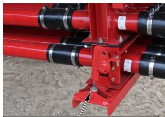
Adjust the latch bolts to obtain a force of 30 lbs (14 kg) to close the Door.
