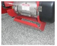
Access cover for incline conveyor cleanout
