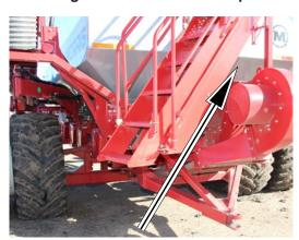
Note: Do not attempt to meter product when fan is not running. Damage to the metering wheels may occur.
