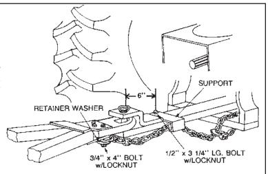
Attach safety chain to the tractor drawbar support or other specified anchor location with the appropriate parts.
