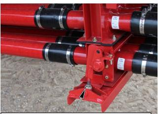
Adjust the latch bolts to obtain a force of 30 lbs (14 kg) to close the Door.
