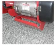
Access cover for incline conveyor cleanout
