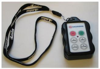
**Meter Shut-Off Remote Control**
