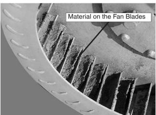
Note: Material build up on the fan blades could cause the fan to be out of balance. The added vibration of the out of balance impeller will reduce the life of the fan components.
