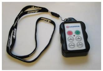
**Meter Shut-Off Remote Control**
