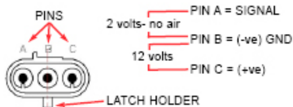
Figure 10-8. Red Collar 3-Pin Weather-Pak Plug
