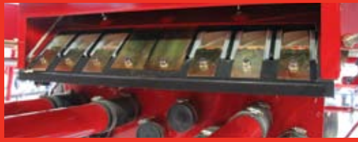
The Post-Drive Transmission uses a positive lock on all drive sprockets to deliver smooth and reliable metering. The positive ground drive from the Air Cart wheel ensures precise product rates at all times.
