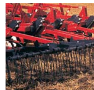
Universal Arm with quick detach pin for changing packers and harrows.
