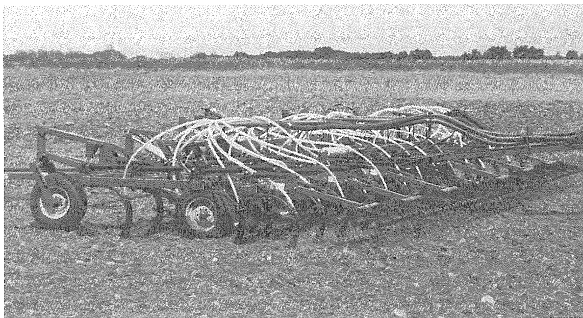
Completed Installation of Hoses on 8900 Floating Hitch Cultivator.
