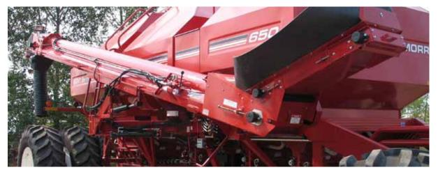
Optional conveyor for 8435, 8630 and 8650 models features a fast 60 bushel per minute loading time with hydraulic remote for convenient one-person operation and requires no clean-out.
