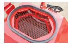
Larger tank openings feature screens (standard) to prevent debris getting into the tanks when filling.
