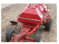
The 8435, 8630 8650 EIGHT Series XL air carts feature a guad steer chassis - using larger tires on the front of the air cart allows you to reduce tire pressure and therefore reduce soil compaction.
