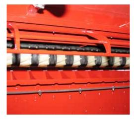
The spiral fluted metering wheel gently rolls a constant flow of product into the air stream, accurately metering grass, canola and other fine seed right up to larger pulse crops and everything in between. This unique design eliminates the need to change wheels and reduces the chance of seed damage and uneven metering.
