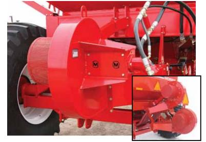
An industrial piston-type hydraulic motor powers a 17" diameter forward curved fan that is 98% efficient. The larger hydraulic lines decrease flow restrictions for less heat build-up under higher fan speeds. A dual fan option for large width seeding tools is available.
