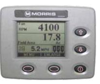
Fan speed, shaft rotation, bin levels, acres seeded and other critical data are at your finger tips with the easy to read Vansco monitoring system.
