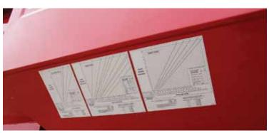
Quickly determine the product rate settings by using the easy to read seed and fertilizer charts located on the side of the air cart (use charts as a guide only). Ensure the proper application rate with a convenient stationary rate check right in your yard.
