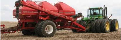
On the tow-between 8650 model the forward axle design provides better weight distribution, lower hitch weight and a tighter turning radius. High floatation, neavy duty dual 800 tires ensures excellent carrying capacity and reduces soil compaction.
