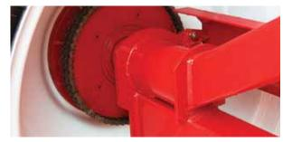
Quick-change sprockets mean simple, reliable adjustments between crops. The posi-drive transmission uses a positive lock on all drive sprockets to deliver smooth and reliable metering. The positive ground drive from the air cart wheel compensates for any changes in ground speed, ensuring precise product rates at all times. Dual speed metering on all three tanks allows you to mix and match product and tanks.
