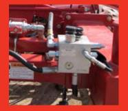
Initial trip out pressure and packing pressure is dialed in and locked on the drill.
