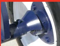
models to protect the hub bearings from mud and debris.
