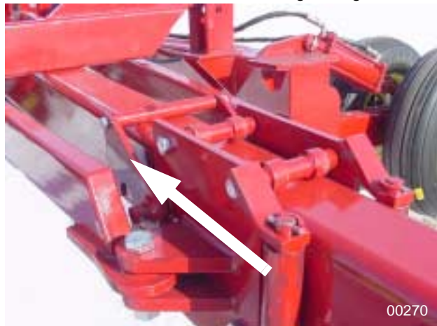
Figure 34 Slide Lock Assembly In Position for Unfolding the Drill
