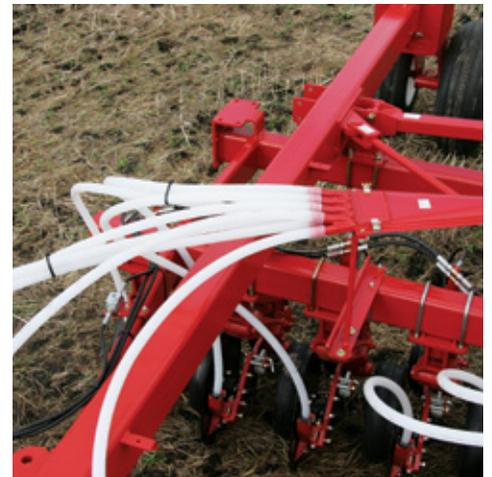
The patented flat fan divider heads maintain the smooth horizontal flow of product as it leaves the primary runs to the divide into each secondary run. This accurate and efficient air delivery system ensures that germination, growth and vigor are protected.
