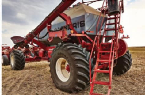
The rear stairway is accessed from the auger side. The retractable section provides a low step height when in use and slides up and locks out of the way for improved ground clearance. The sliding section has two larger gas cylinders that help lift and hold the stairs until locked in position. A spring-loaded pin reduces latch time.
