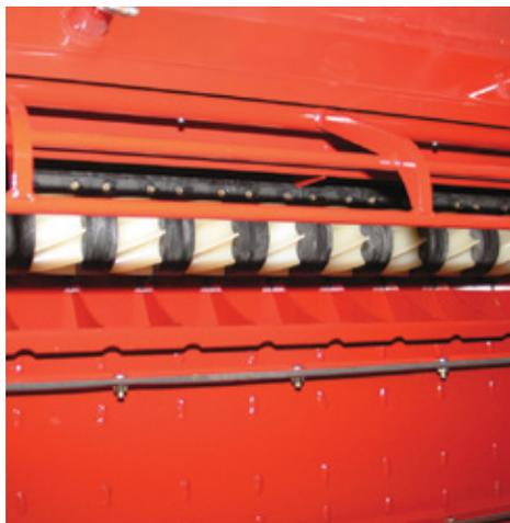
The time-proven spiral fluted metering wheel is the center of the metering system. The spiral flute provides a continuous flow of product into the air stream. The meter-bodies include single person operation of the inspection and calibration left side access doors. Calibration doors speed up calibrating time because the operator does not have to pick up parts from the ground. The 9800 and 91000 metering bodies accommodate up to 10 metering wheels.
