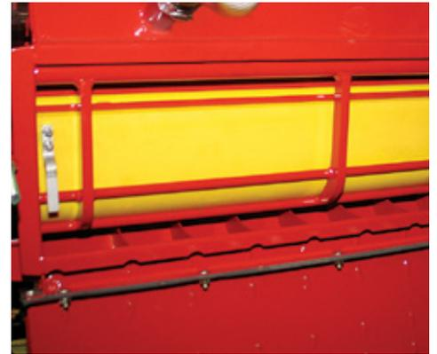
All-in-one seed plates save time, one quick change lets you accurately meter fine, medium or coarse products. The operator can quickly inspect the seed-plate in each meter-body.
