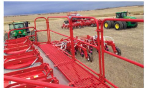
Filling of the tanks is made easier by designing the tank lids to be closer together. With the optional hydraulic assist the operator can use the wireless controller to position the spout on the auger/conveyor without moving the hopper from the unloading area or climbing down from the air cart. The lid design incorporates a gas cylinder to assist the operator when opening and closing the tanks. The handle
