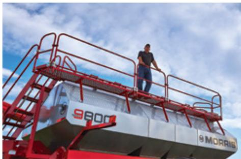
The walkway improves access to the tank lids. Handrails around the walkway platform and down the stairway provide excellent protection for a secure and safe work area. The walkway is positioned to allow the operator more room to work and avoid dust when filling the tanks.
