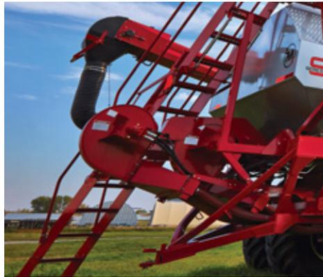
An industrial piston-type hydraulic motor powers the 17" diameter forward curved fan and large hydraulic lines decrease flow restriction for less heat build up under higher fan speeds. A dual fan option is available for large width seeding tools.
