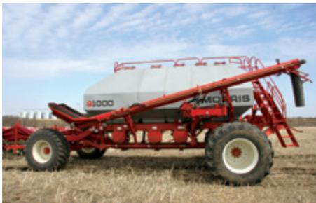
Left side auger/conveyor for easier access when filling. A 6-function wireless remote included with the hydraulic assist options reduces operator fatigue. The lanyard allows the operator to safely use two hands when necessary. New transmission covers for added operator safety on all carts. Quick-detach straps on the standard drive allow easy access to the quick-change sprockets.
