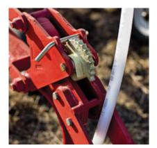
The one-to-one parallel linkage maintains а constant opener angle relative to the soil and opener depth relative to the packer wheel throughout its range of travel. The opener can contour up 25 cm (10 inches) and down 18 cm (7 inches).
