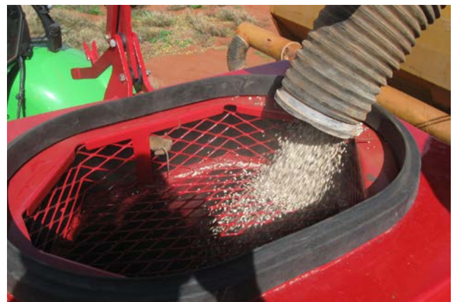
Tank Screen to filter debris
