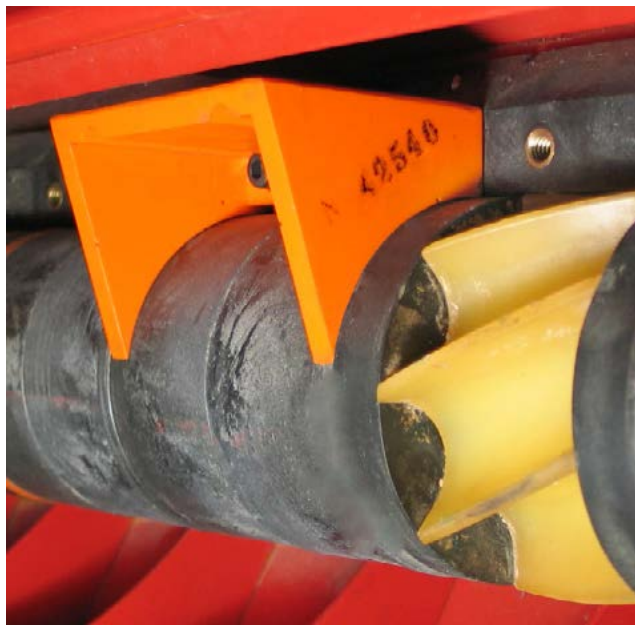
Correctly Installed Blank Off
