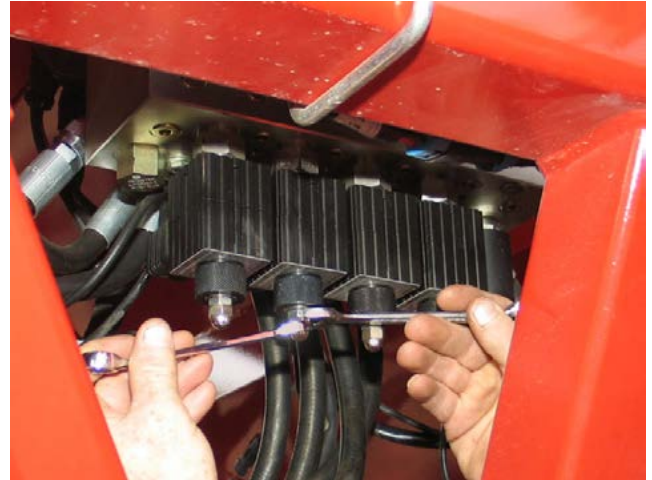
Remove Cap Nut and Loosen Jam Nut
