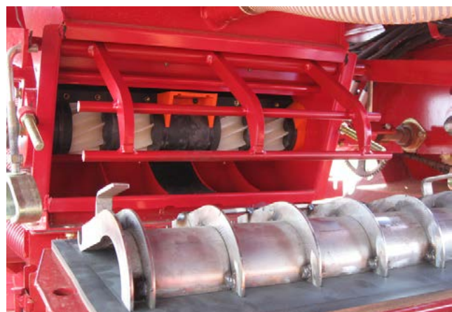
Inspect Metering Body
